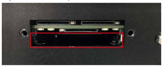
Step 4 Insert CFast card and push to lock.
