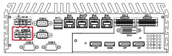
It is a 5-pin power-on or power-off switch through Phoenix Contact terminal block. You could turn on or off the system power by using this contact. This terminal block supports dual function of soft power-on/ power-off (instant off or delay 4 second), and suspend mode.
