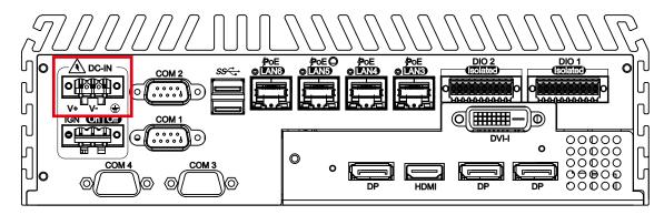
This system supports 10V to 36V DC power input by terminal block in the rear side. In normal power operation, power LED lightens in solid green and supports up to 80V surge protection.
