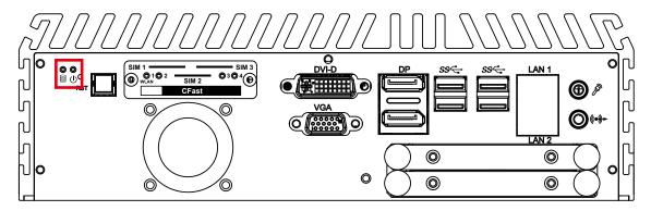
HDD LED/ Yellow: A Hard Disk/ CFast LED. If the LED is on, it indicates that ECS-9700/9600 GTX950 storage is functional. If it is off, it indicates that the system's storage is not functional. If it is flashing, it indicates data access activities.
