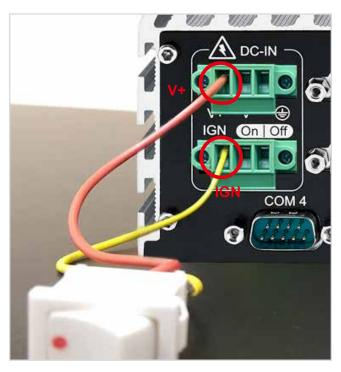
For testing purpose, you can refer to the picture above to simulate ignition signal input controlled by a latching switch.
