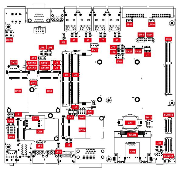
The figure below is the top view of ECS-9700/9600 GTX950 board, and it shows the location of the jumpers and the switches.
