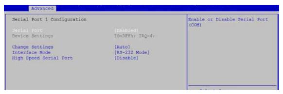
Figure 4-3-6-2: Serial Port Settings
