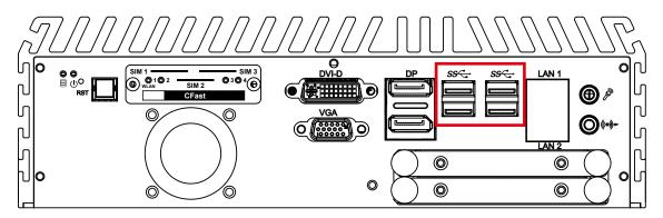
There are 4 USB 3.0 connections available supporting up to 5GB per second data rate in the front side of ECS-9700/9600 GTX950. It is also compliant with the requirements of Super Speed (SS), High Speed (HS), Full Speed (FS) and Low Speed (LS).
