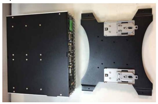
**Step 2** Take ECS-9700/9600 GTX950 and Din Rail Kit and fasten four KHS#6-32 screws in the four marked corners.
