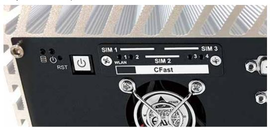
**Step 2** Before Inserting CFast & SIM Card, make sure ECS-9700/9600 GTX950 power is not plugged.
