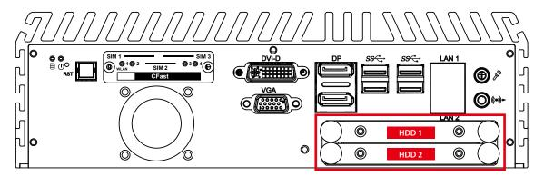
There are 2 front-access 2.5" SSD/ HDD trays in the front side of ECS-9700/9600 GTX950. Just trigger to open the SSD/ HDD tray, up to 8TB is available.
