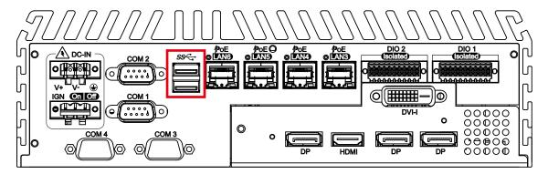
There are 2 USB 3.0 connections available supporting up to 5GB per second data rate in the front side of ECS-9700/9600 GTX950. It is also compliant with the requirements of Super Speed (SS), High Speed (HS), Full Speed (FS) and Low Speed (LS).
