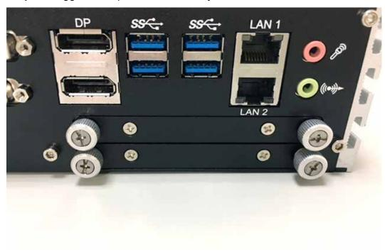
**Step 2** Insert 2.5" SSD/HDD in the tray and fasten two F-M3x4 screws.
