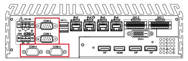
Serial port 1 to 4 (COM 1 to 4) can be configured for RS-232, RS-422, or RS-485 with auto flow control communication. The default definition of COM 1 and COM 2 is RS-232. If you want to change to RS-422 or RS-485, you can find the setting in BIOS.
