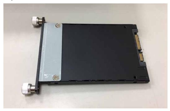
**Step 4** Installing SSD/HDD.
