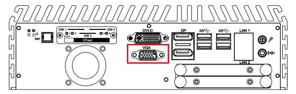
The VGA connector on the front panel supports VGA display. This VGA connector comes from eDP and the VGA output mode supports up to 1920 x 1200 resolution.
