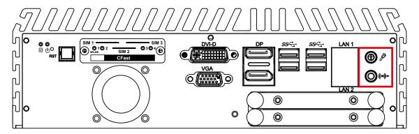
There are 2 audio connectors, Mic-in and Line-out, in the front side of ECS-9700 /9600 GTX950. Onboard Realtek ALC892 audio codec supports 5.1 channel HD audio and fully complies with Intel® High Definition Audio (Azalia) specifications.
