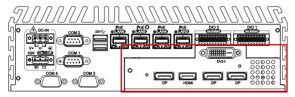
You could have 4 independent displays as your wish from these 5 display ports. Also, you could have four 4K resolution displays, the 3 DisplayPort and a HDMI, from these 5 ports.
