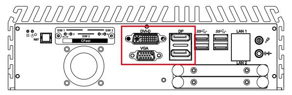
You could have 3 independent displays as your wish from these 4 display ports. Also, you could have two 4K resolution displays, the 2 DisplayPort, from these 4 ports.
