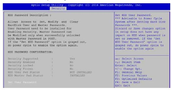
Figure 4-5-1: HDD Security Settings
