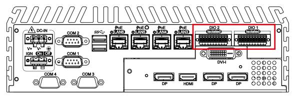
There is a 32-bit (16-bit DI, 16-bit DO) with 2 DIO connectors in the rear side. DI/DIO supports NPN(sink) and PNP(Source) mode, and each DI channel is equipped with a photocouper for isolated protection. Each DO with isolator chip is configured by a Jumper for each DIO connector.
