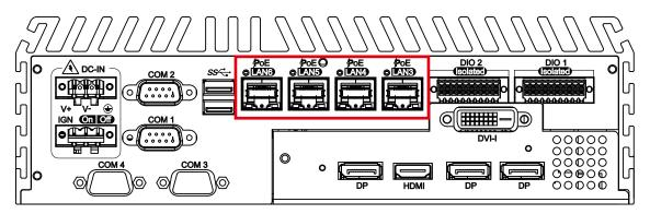
There are quad 8-pin PoE RJ-45 jacks supporting 10/ 100/1000 Mbps Ethernet connections in the front side. Powered by Intel I210 Ethernet engine. When both LAN 1 and LAN 2 work in normal status, iAMT 11.0 function is enabled. Each PoE supports 30.4W
