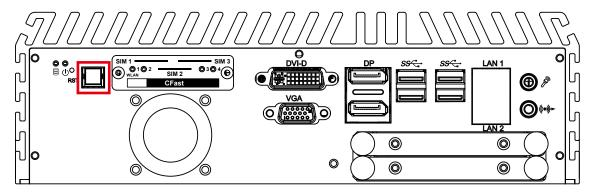
The Power Button is a non-latched switch with dual color LED indications. It indicates power status: S0, S3 and S5. More detail LED indications are listed as follows:
