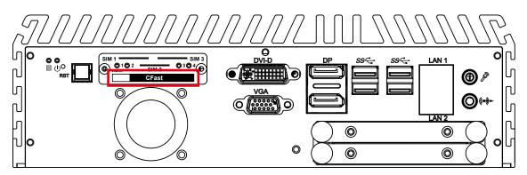
There is a CFast socket on the front panel supporting Type-I/II Compact Flash card. It is implemented by a SATA III Port from CM236 PCH. Be sure to disconnect the power source and unscrew the CFast socket cover before installing a CFast card. The ECS-9700 does not support the CFast hot swap and PnP (Plug and Play) functions. It is necessary to remove power source first before inserting or removing the CFast card.
