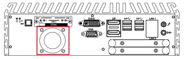
There is a system FAN on front side for airflow direction outward. You can adjust the FAN Speed from Vecow BIOS Setting. (refer to 4.3.7\_Hardware Monitor\_FAN PWM Value)
