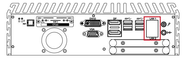
There are dual 8-pin RJ-45 jacks supporting 10/ 100/1000 Mbps Ethernet connections in the front side. LAN 1 is powered by Intel I219 Ethernet Phy and LAN 2 is powered by Intel I210 Ethernet engine. When both LAN 1 and LAN
