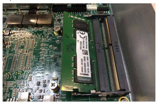
**Step 2** Make sure the RAM module is locked by the memory slot.
