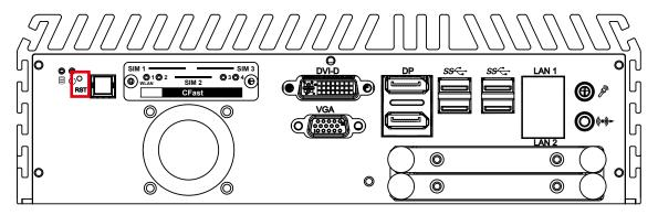
It is a hardware reset switch. Please use this switch to reset ECS-9700/9600 GTX950 without power off. Press the Reset Switch for a few seconds, and then reset will be enabled.
